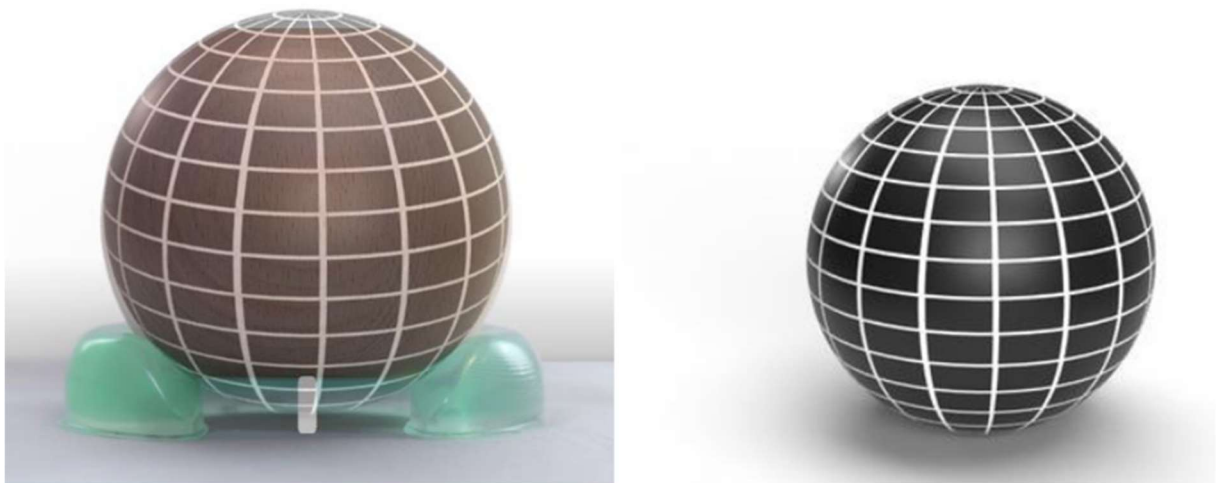
Figure 2: Test arrangement with head support ring (Setting A, left) and without head support ring (Setting B).
