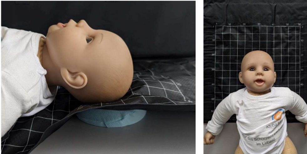
Figure 3: Experimental set-up for measuring the pressure load. Shown is the test set-up for measuring the pressure between the head model and the gel cushion or the flat base is shown.
